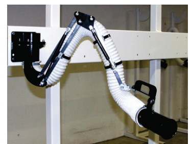
Open extraction hood (e. g. for die change)
